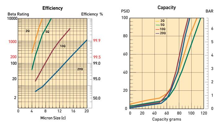
Results typical from Multi-pass tests run per test standard ISO 16889 @ 50 gpm to 100 psid terminal - 10 mg/L BUGL Refer to Appendix for relationship to test standard ISO 4572.
