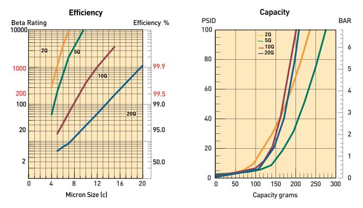
Results typical from Multi-pass tests run per test standard ISO 16889 @ 80 gpm to 100 psid terminal - 10 mg/L BUGL Refer to Appendix for relationship to test standard ISO 4572.
